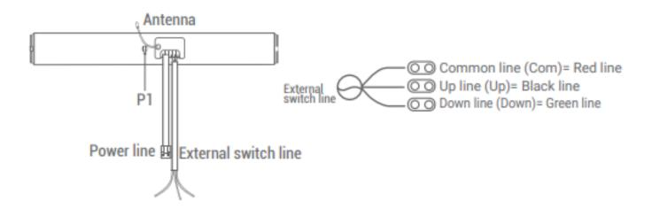
The BJE24DD motor is ideal for **projects** with indoor shading. Because the motor is equipped with an extra dry contact wire, it is very suitable for connection to home automation systems and building management systems. In addition, the motor is **easy to install** due to the bi-directional radio protocol.
