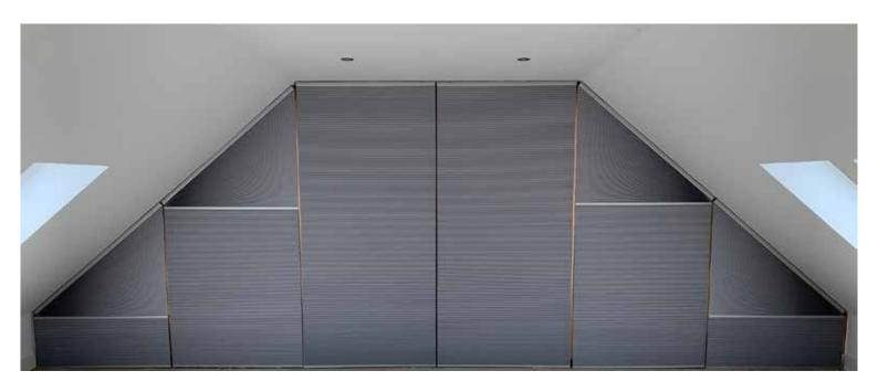
BREL HOME is continuously developing new motors. The BJE24TR was made in collaboration with **Benthin**. This motor has been specially developed for **angled windows**, so that they can be fitted with pleated blinds. The Triangle motor ensures that the intermediate bar of the pleated blind first goes down until it is horizontally. Then the bottom bar will drop to the end position. This prevents the angled pleated blind from getting stuck in the window.
